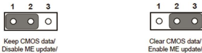
**Figure 3.1 ECU-579 Jumper position indication**
